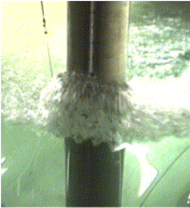
Figure 10. Flow past immersed column in water model
